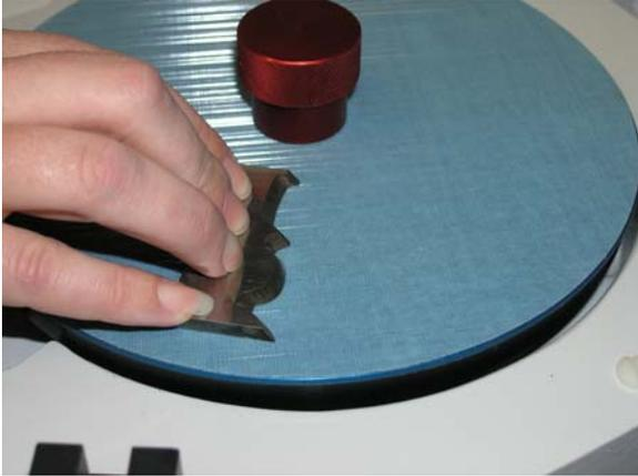
Hold the back of a profile knife flat on the abrasive
